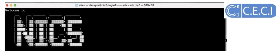
the new (January 2021) ULiege/CECI cluster, featuring: 70 nodes with two 32 cores AMD EPYC Rome 7542 cpus at 2.9 GHz and 250 GB of RAM, 3 nodes with 1 TB of RAM, 520 TB of fast BeeGFS \$GLOBALSCRATCH and a 100 Gbps Infiniband HDR interconnect (blocking factor 1,2:1), for a total of 4672 cores. Max walltime is 2 days. See also https://www.campus.uliege.be/nic5
